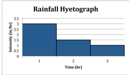
2. Calculate the area under the hydrograph to get the total volume of all runoff:
