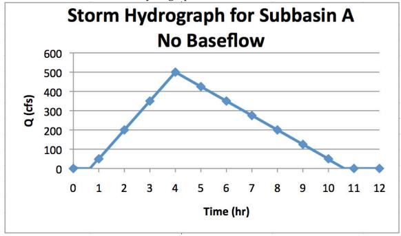
If you just generate this as a line chart then hours 0 and 1 as well as 10 and 11 will directly connect. This flares out the bottom of the triangle and is not accurate. The way to get around this is to create two extra points (.66 hr, 0 cfs) and (10.66 hr, 0 cfs) and then graph the whole thing as a scatter plot.
